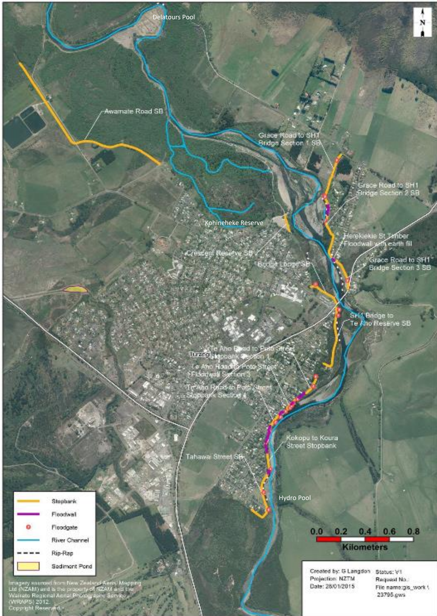
Figure 1: Tongariro River Flood Control Scheme
